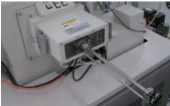
150mm diameter specimen exchange chamber for large/multi sample observation
