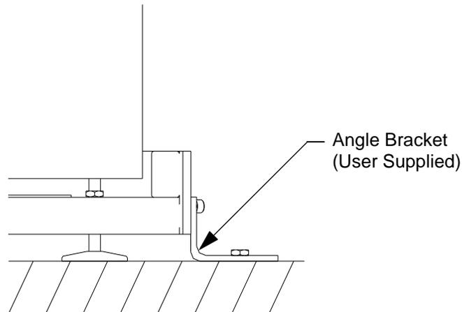
Figure 3-3: Seismic Bracket Mounting
