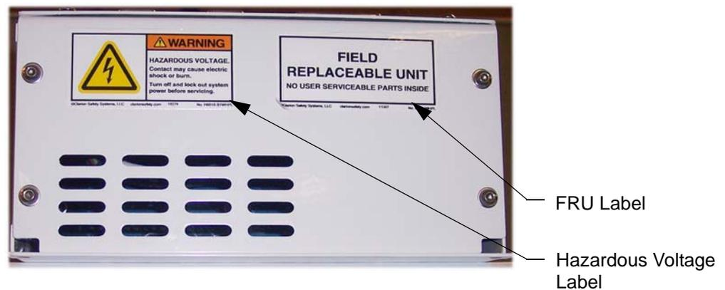
Figure 2-5: Label Locations on the Safety Hub
