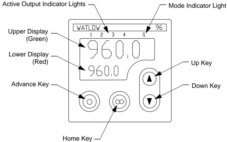
Figure 5-14: Temperature Controller
