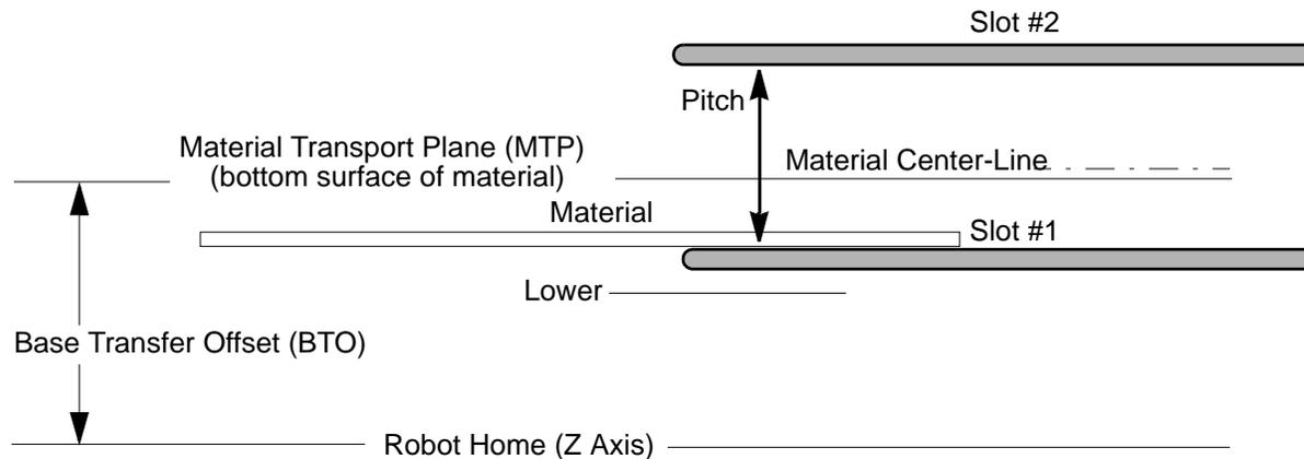
Figure 5-3: Robot Z-Axis
