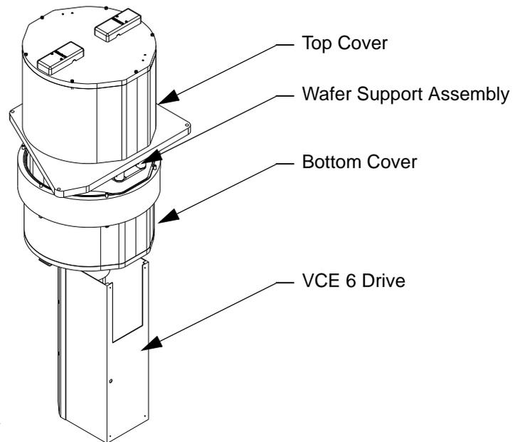
Figure 5-9: Batch Load Lock
