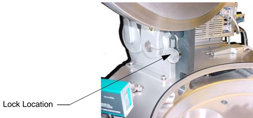
Figure 2-7: Installing Lid Lockout/Tagout Device
