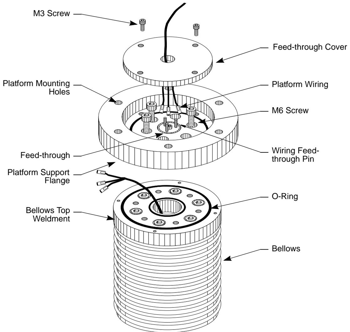
Figure 6-1: Platform Support Flange and Bellows
