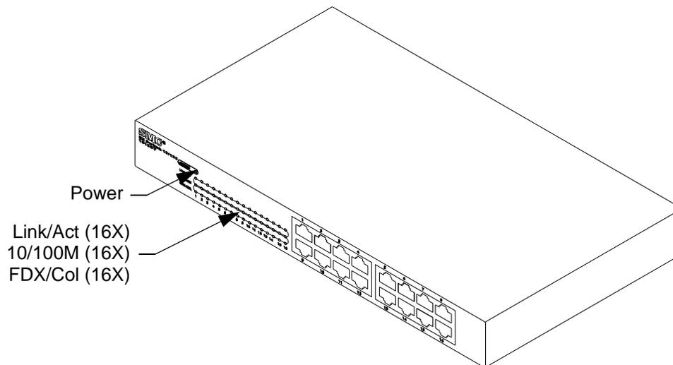
Figure 5-15: Ethernet Switch Module - Controls and Indicators
