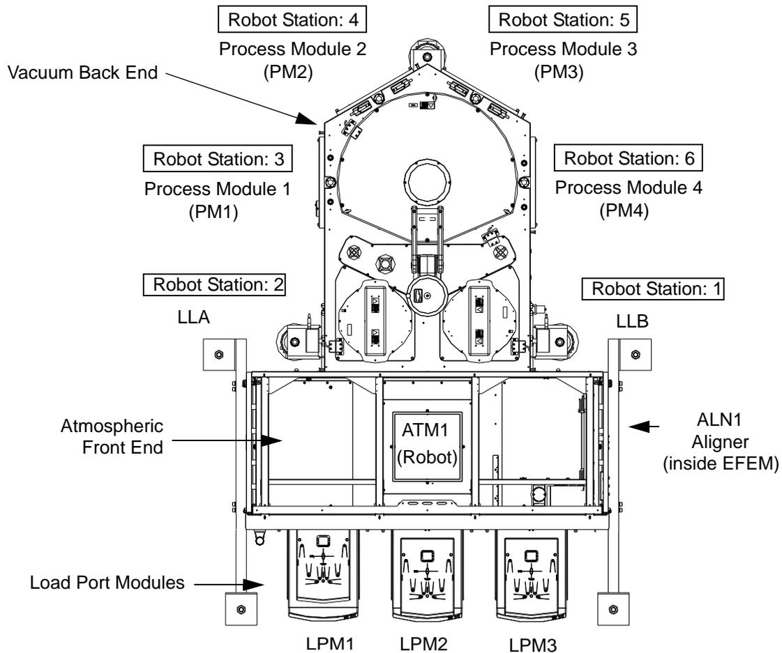
Figure 5-2: Station Assignment Example (G2 6000 shown)
