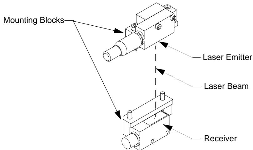
Figure 5-16: Wafer Centering Sensor
