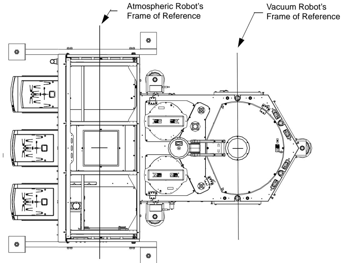
Figure 5-4: Frames of Reference (Typical System)
