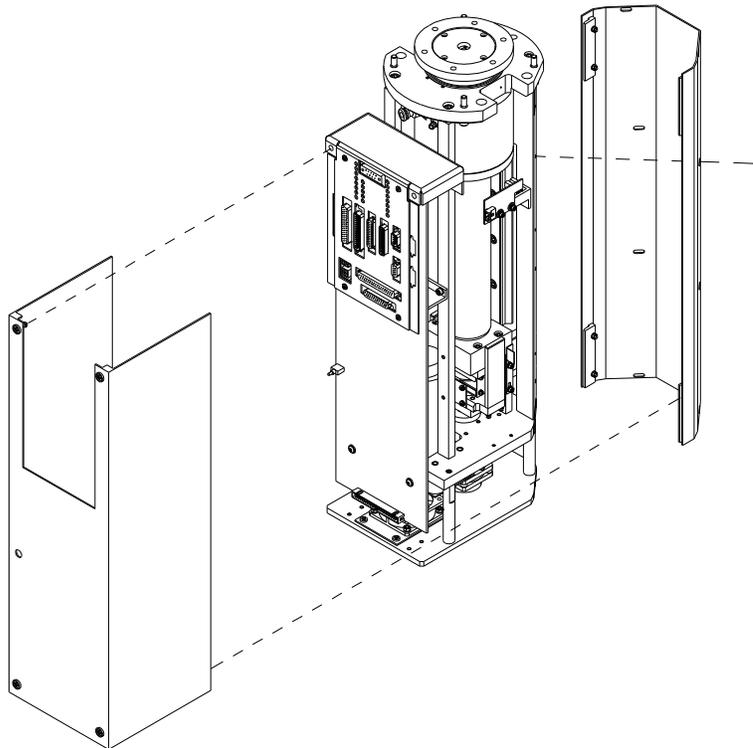
*Figure 6-2: Batch Load Lock Drive Cover Removal*
