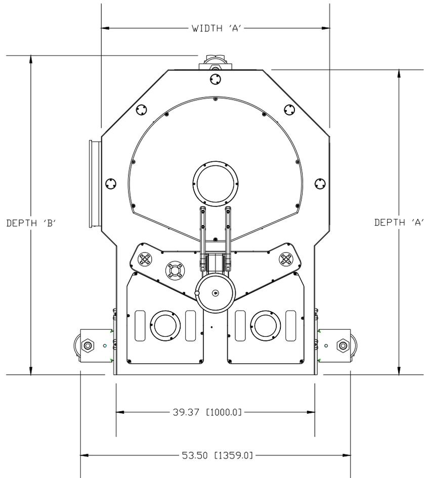
Figure 1-2: Gemini 2 Back End Dimensions - Typical
