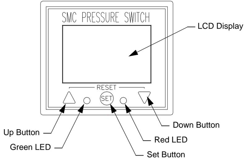
Figure 5-17: N2 Pressure Switch - Controls and Indicators
