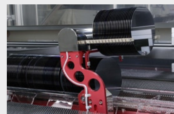
Fully automated cassette-to-cassette production up to 200 wafers per tube
